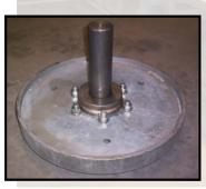
24" Traction wheel with Dodge #70 6 bolt Bearing assembled
